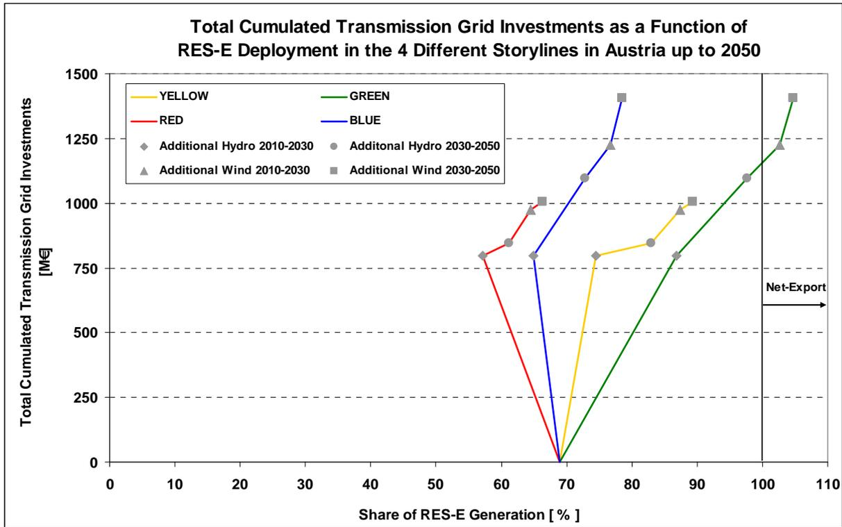
**Figure 4.12 Total cumulated transmission grid investments as a function of RES-E deployment in the four different storylines in Austria up to 2050**
