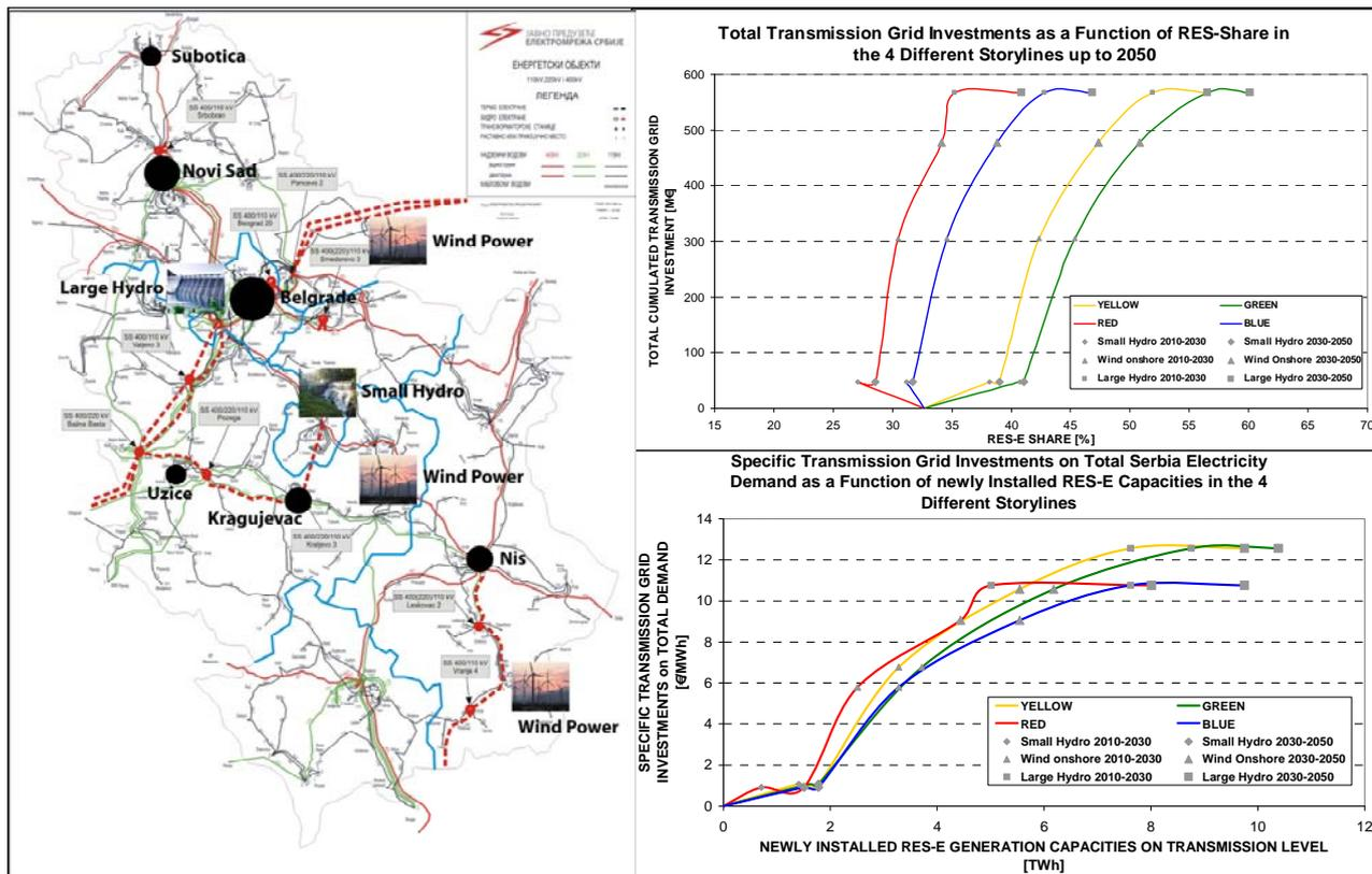
**Figure 4.11 Spatial dispersion of RES-E potentials, load centers and transmission grid routes in Serbia (left); total transmission grid investments as a function of RES-E share (upper right) and specific transmission grid investments as a function of newly installed RES-E capacities (lower right) in the four different storylines in Serbia up to 2050**
