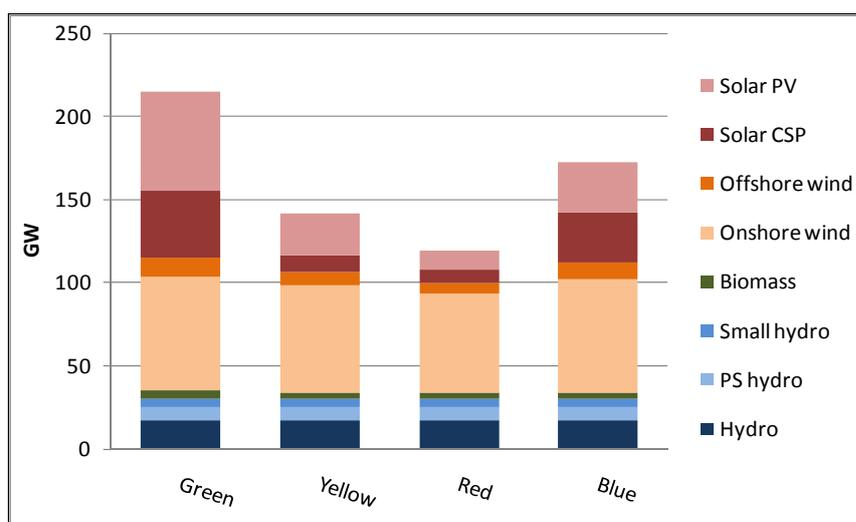
**Figure 4.7 Installed RES-E capacities in Spain in the four different storylines up to 2050**
