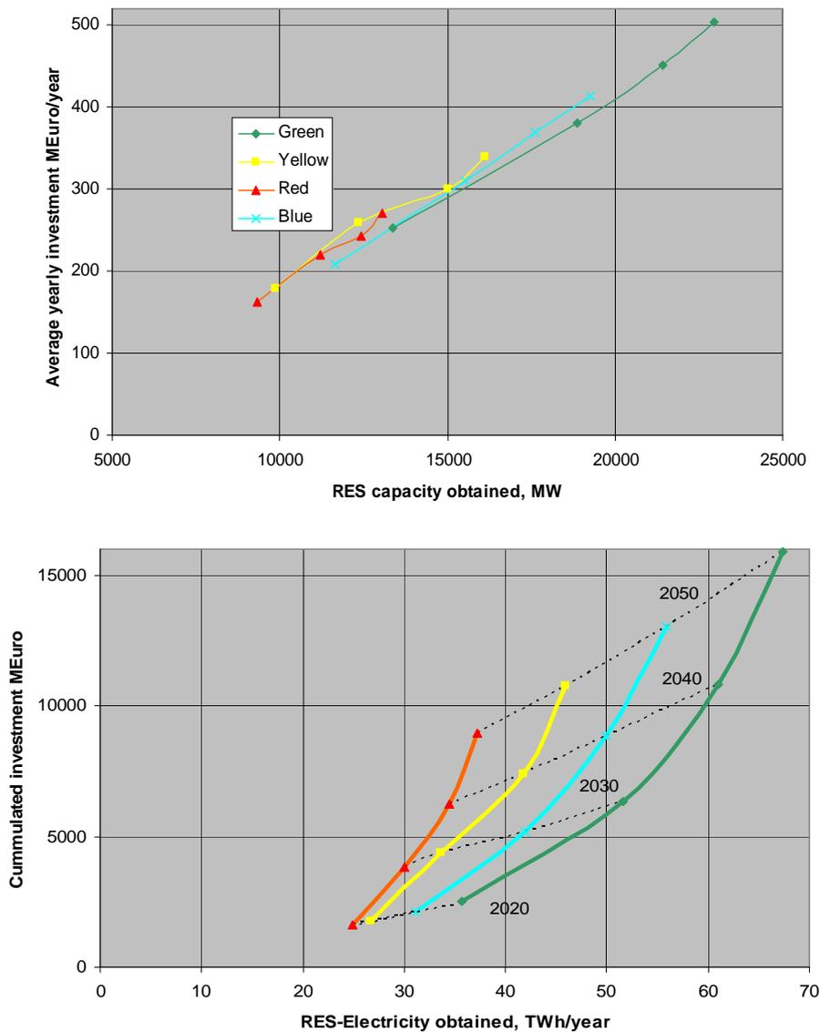
**Figure 4.6** Average annual investments in the transmission grid versus RES-E capacity expansion (top); cumulated transmission grid investments versus annual RES-E generation obtained for different years in the future up to 2050 (bottom)
