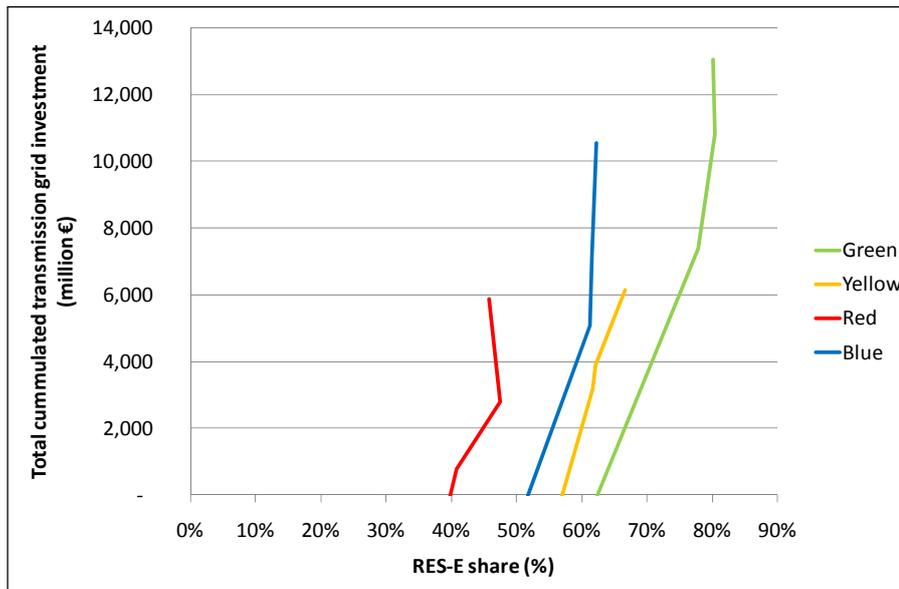
**Figure 4.8 Total cumulated transmission grid investment cost over RES-E penetration in the four different storylines up to 2050**
