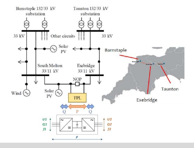
Dynamically controlled distribution grids by means of power electronics allow a better balancing and utilization of existing infrastructure
