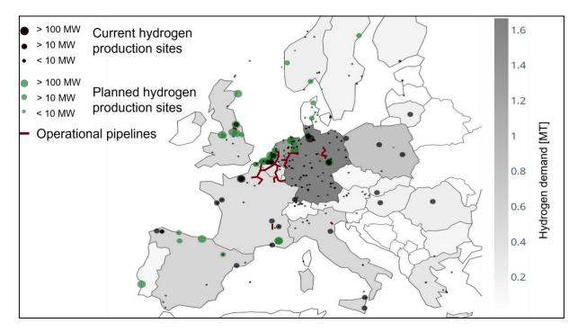
**Figure 2:** The selected locations of the current and planned centres of hydrogen production in Europe and existing pipelines (Source: own visualisation, based on IEA (2021)<sup>7</sup>, FCHObservatory (2022)<sup>8</sup>, FCHObservatory (2022).<sup>9</sup>
