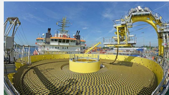
Cable laying vessel © Caley Ocean / Cable Turn Table © VBMS
