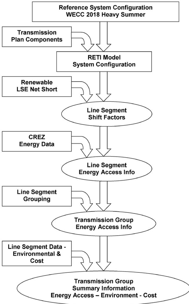
Fig. 2. Flowchart for RETI Conceptual Plan Assessment.
