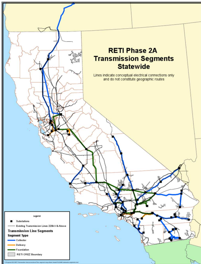
Fig. 3. Conceptual Plan Line Segments.
