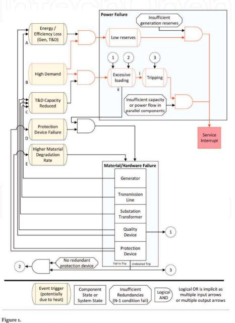
Fault tree from heat wave to service interruption.
