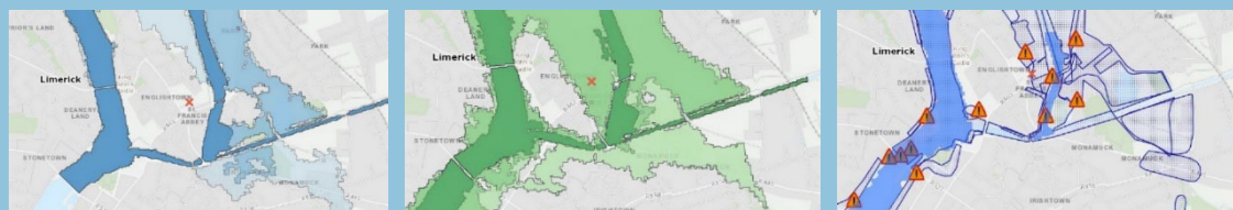
Figure 45: a) River flooding, b) Coastal flooding, c) Previous flood records
