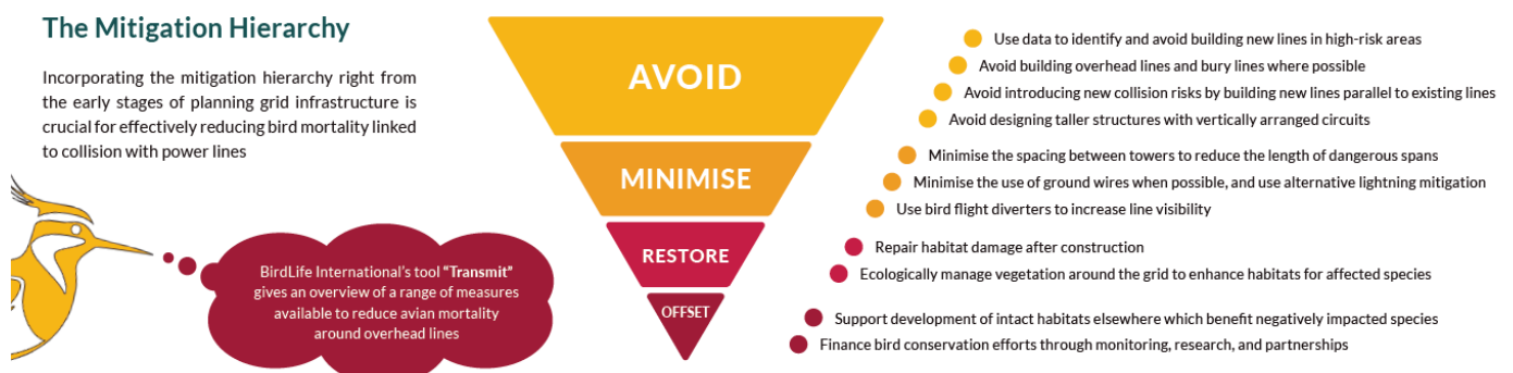
Figure 3: The above model from the Brochure will not always be practical, (i.e. ground wire removal) and is only offered as a guide. When an action is not possible to follow due to conflicting priorities, the emphasis of the design team should always shift to mitigation steps first, and if this mitigation is not possible, then to restoration, offset etc. Source: RGI
