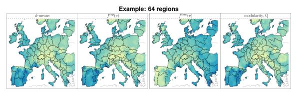
avg. annual capacity factors (wind and solar combined), avg. at 8 o'clock for  $f^{\text{time}}$
