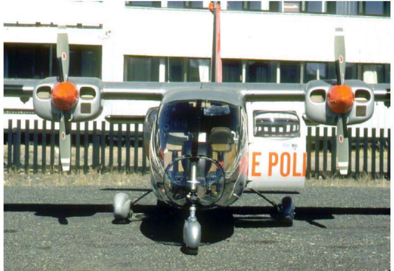
Figure 1. Partenavia P-68 Observer aircraft. Note the plexiglass nose for pilot and front seat observer, and bubble windows on both sides of the aircraft in the rear passenger panels (see on open door to right).
