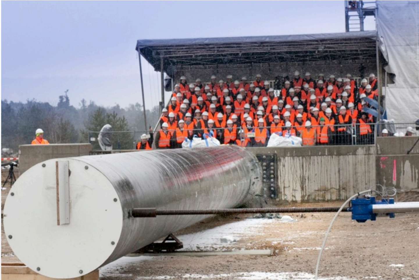
Pole Bending Test – UHPC, Load 80 tons
