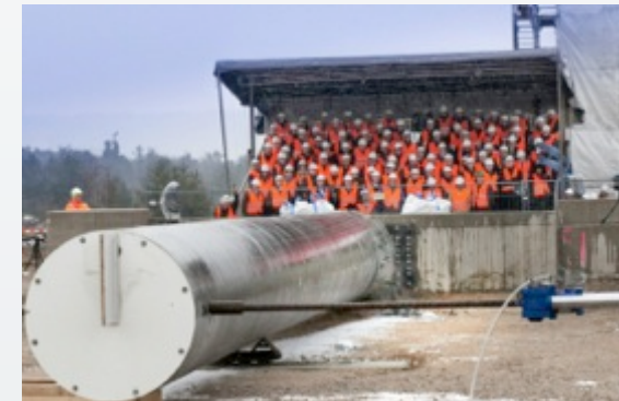
Pole Bending Test with the equivalent of 80t tractive force
