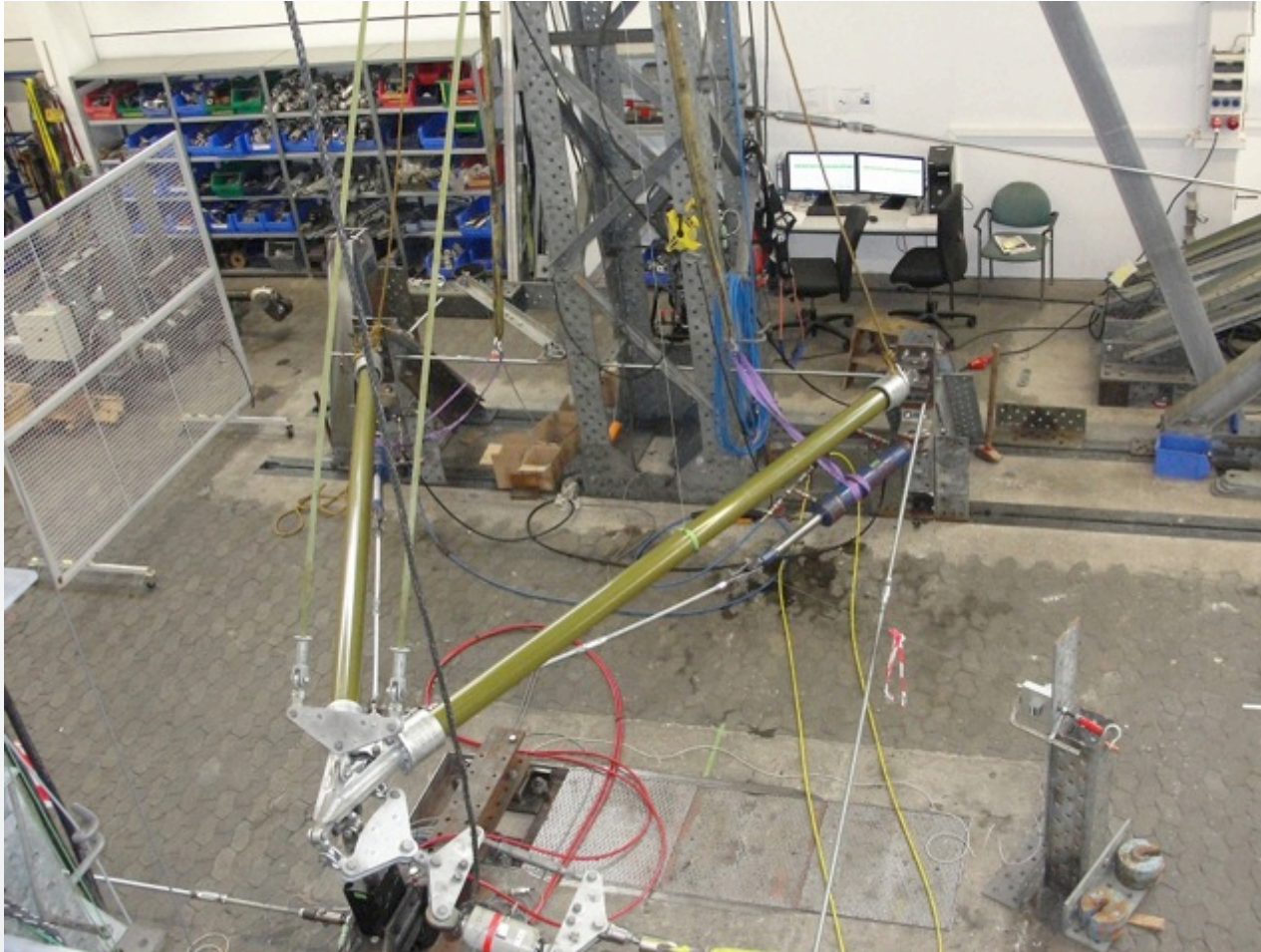
Full Scale Testing of Fiberglass Isolators
